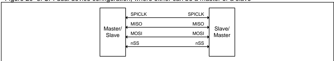
Figure 20–3. SPI dual device configuration, where either can be a master or a slave
